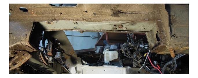
Prepare the area for welding – clean and grind down the spot welds.
