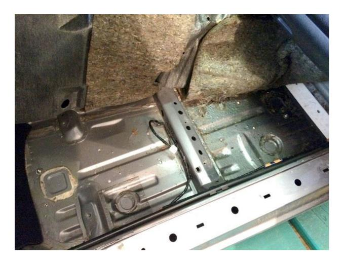
Under the car loosen the brake and fuel lines from the holders that need to be removed completely. Separate the plastic part from the metal part, dispose of the metal and clean the plastic. Then mount the plastic holder to the new mount provided with our rails (photo).
