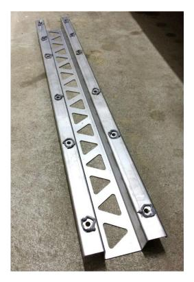
After the paint has dried off, put some filler or silicone around the holes on rails (or both – on rails and on floor) to make sure it will seal properly (photo). Install the rails and tighten the nuts – we advise to do the tightening in two stages. There is no recommended torque but we're confident the stainless steel bolts and nuts can handle a reasonable amount (applied by hand), but there's no need for anything crazy.
