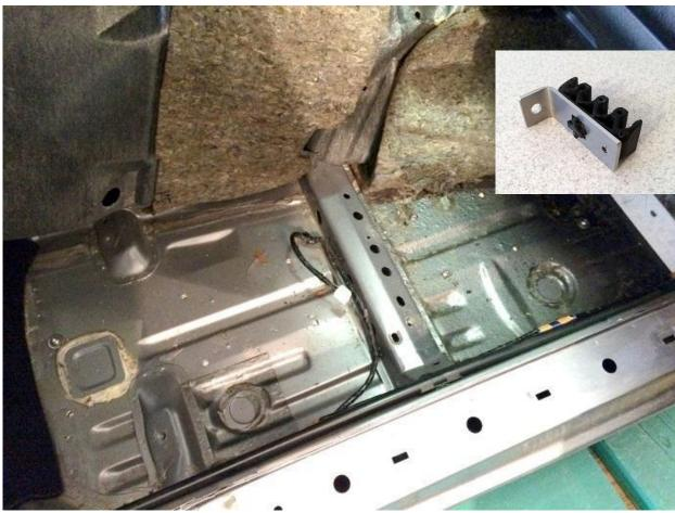
Under the car loosen the brake and fuel lines from the holders that need to be removed completely. Separate the plastic part from the metal part, dispose of the metal and clean the plastic. Then mount the plastic holder to the new mount provided with our brace (photo).
